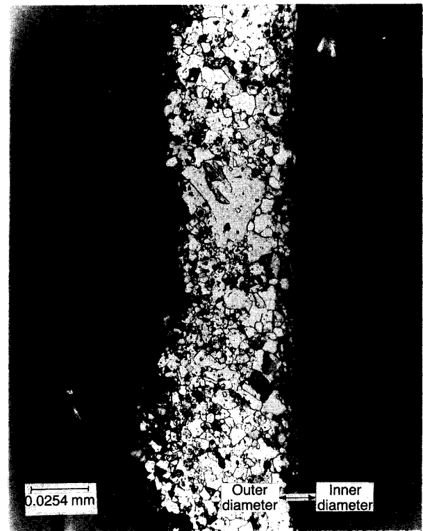
Figure 4 Photomicrograph of TMI-1 specimen G3 showing single layer of large grain intermixed with small grain.
