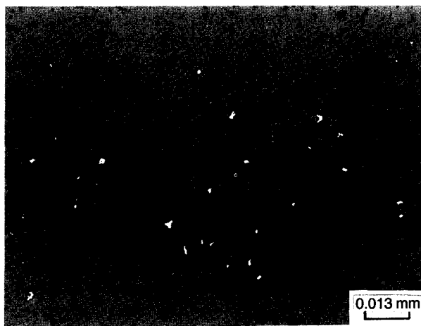
Figure 3 Oconee-2 magnetite in the as-polished condition sectioned parallel to the tube axis. White areas are copper-coloured particles.
